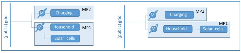
Setup of Household with a Charging point for an electric vehicle and Solar cells.
