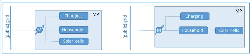
Traditional setup of Household with a Charging point for an electric vehicle and Solar cells. In this case all covered in one Metering Point, where the total consumption / production is netted.
