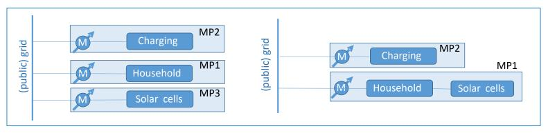
Setup of Household with a Charging point for an electric vehicle and Solar cells.
