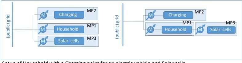
Setup of Household with a Charging point for an electric vehicle and Solar cells. In this case covered in three Metering Points, where in the series case the measurements of consumption / production of the household and the Solar cells is dependent (and may not be allowed).
