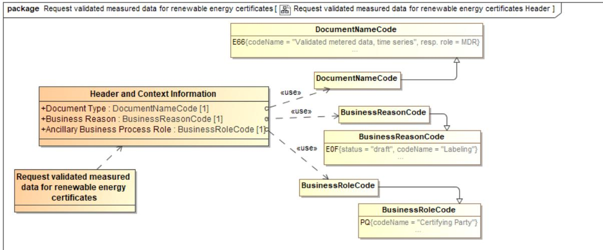
Figure 6 Header and Context Information (class diagram): Request validated measured data for renewable energy certificates
