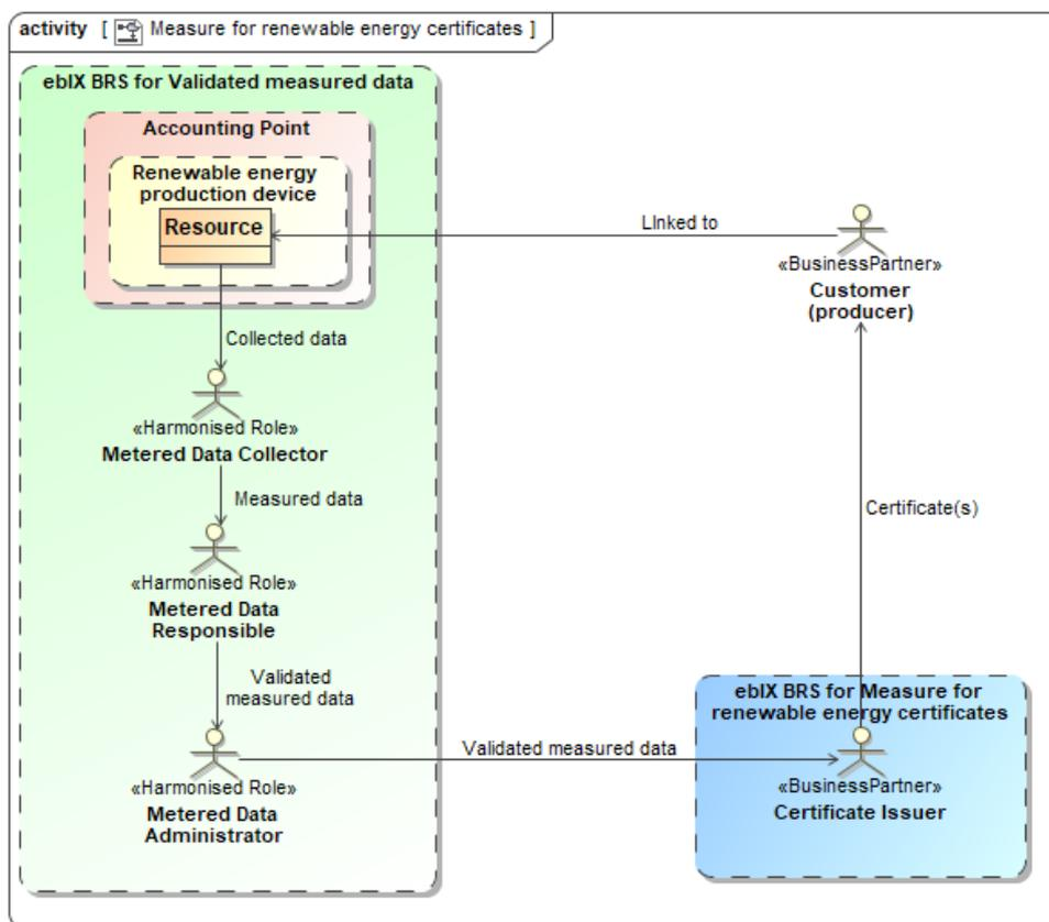
Figure 1 Activity diagram: Overview of Measure for renewable energy certificates
